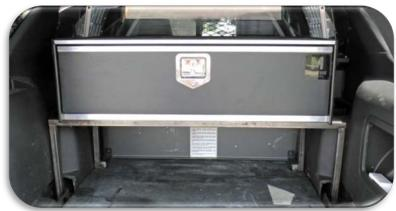
1 Set the box on the stand so that the mounting holes on the side of the box and the frame line up
