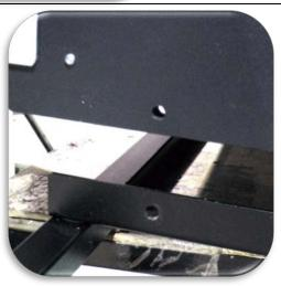
$2\,$  Insert the included 1/4-20 by 1" hex bolt through the angle bracket and into the HDP box and secure with nut and lock washer
